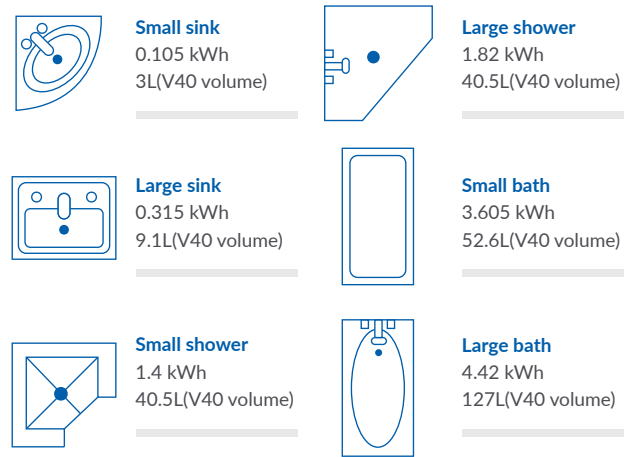
Image 4: Assigned Energy and Hot Water Use at a mixed outlet temperature of 40°C for different end uses from BS EN 16147: 2017
